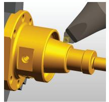
turned diameters, bores, grooves and faces. This function is useful where a turned component needs some elements to be finished turned, and others to be left a grinding allowance for subsequent machining or heat treatment. Most systems on the market today will only allow you to set a constant offset, where as Edgecam gives the user full control over offsets for each individual element on the turn feature.
