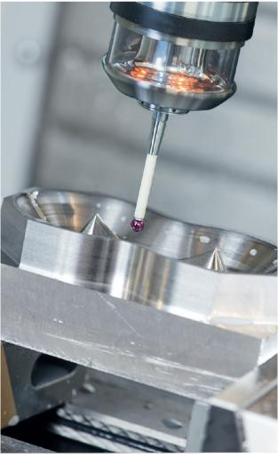
Edgecam Inspect offers the CAM user a robust, user friendly set of tools for creating measurement cycles, which can greatly reduce setup time and error and provide reliable in-process measurement results.
